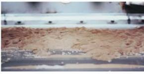
The damp material is plugging up the screening surface by adhering to the wire mesh, reducing the efficiency, capacity and overall performance of the screener.
